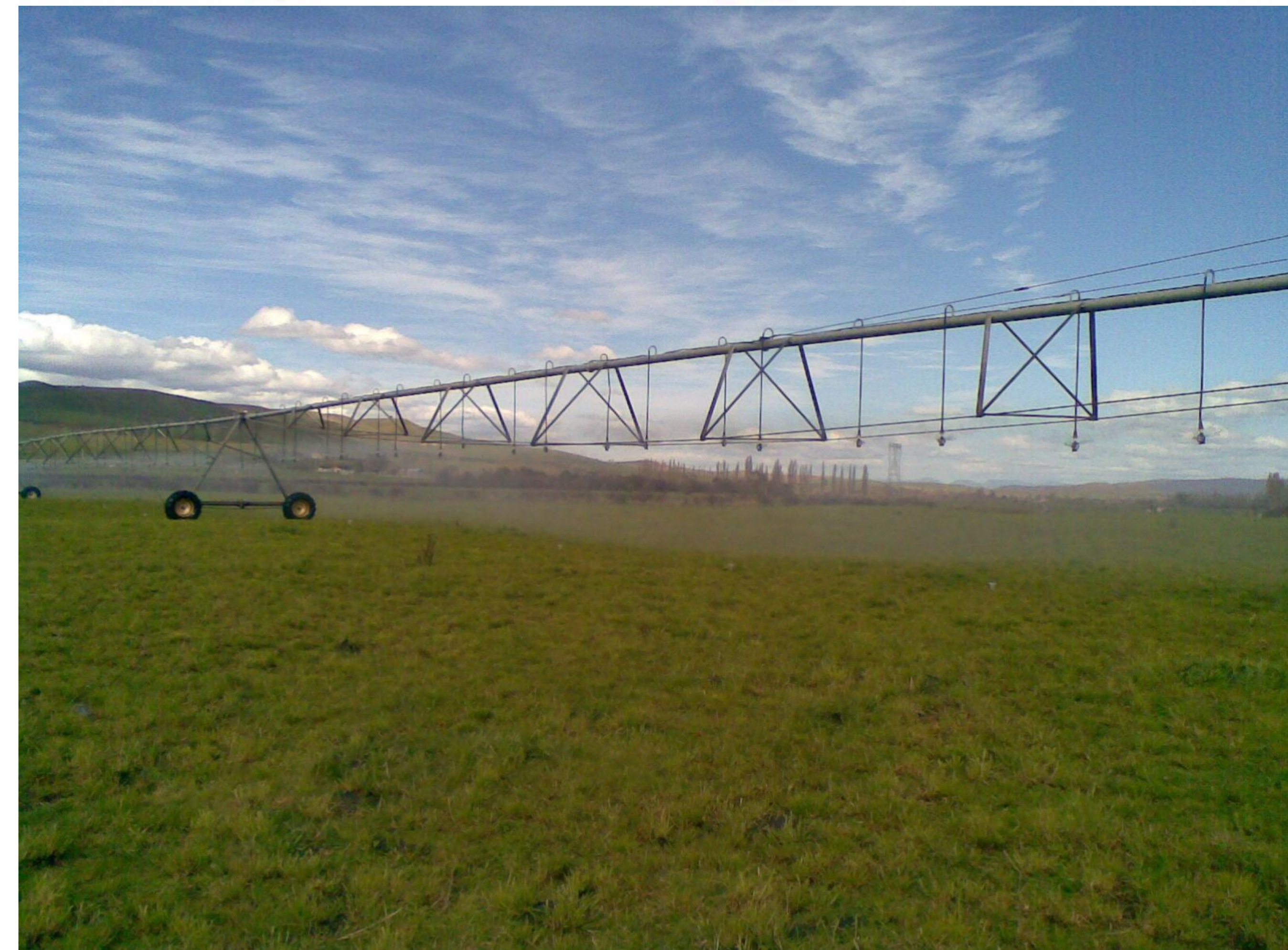
Plate 1. Measuring the distribution uniformity (DU) of centre pivot irrigator
