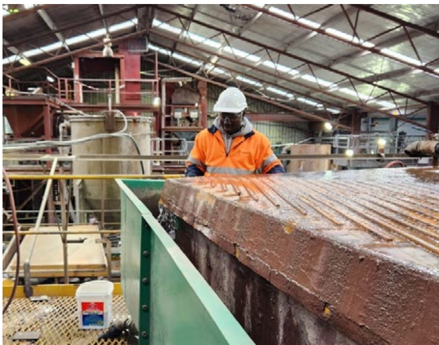
Musa Emmanuel Dogara undertaking gravity beneficiation using a shaking table at the Kara mine in western Tasmania as part of his PhD research.
