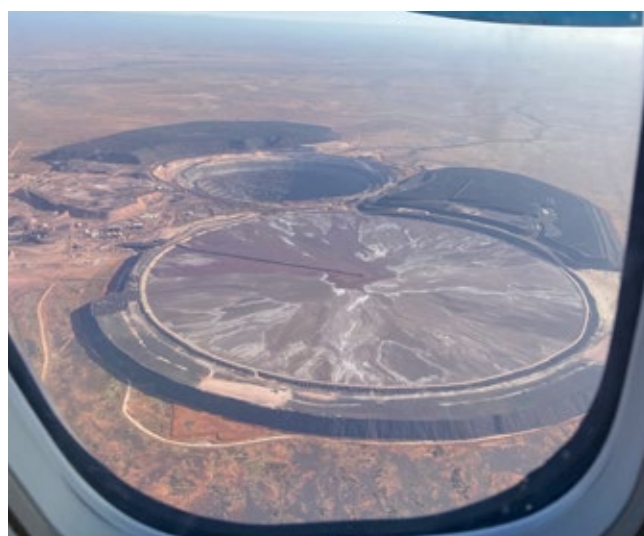
South Australia: Aerial shot of the Prominent Hill mine complex (view to the north), including the open pit, waste dumps and tailings dam (large circle in the foreground). This iron oxide copper-gold (IOCG) deposit is owned and operated by BHP, who are sponsoring Dr Jeff Steadman's IOCG 3 project.
