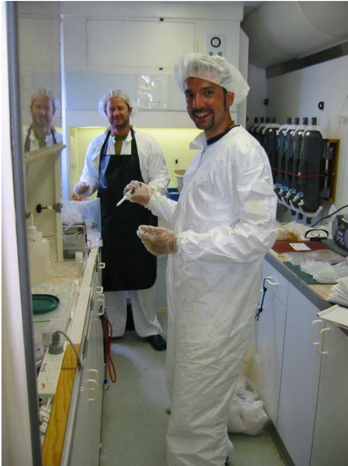
Left. Filtration and analysis for dissolved iron inside a portable clean container van located on the deck of the research vessel Weatherbird II .
