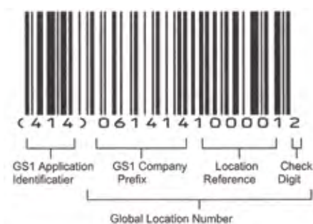
Figure 45. An example of a GLN in a GS1-128 barcode. The application Identifier (414) indicates that the GS1 Application Identifier data field contains the Global Location Number (GLN) of a physical location. The GS1 Company Prefix may be of variable length. The Serial reference varies on length as a function of the GS1 Company Prefix Length. The Digit is calculated on digit number used to ensure data integrity.
