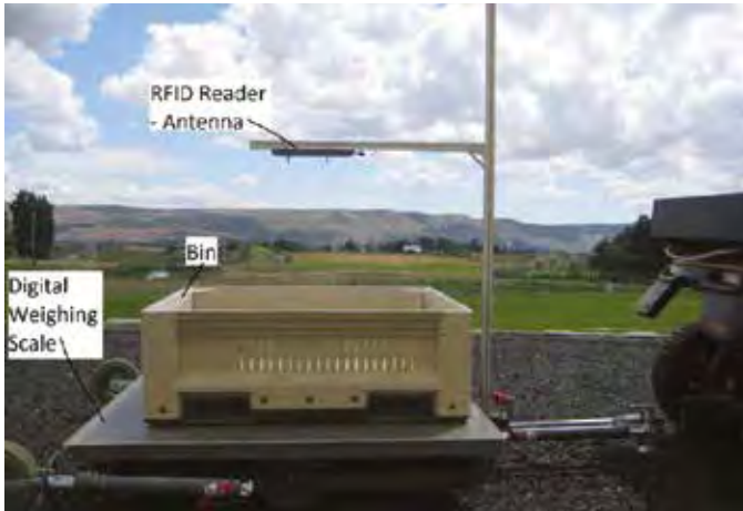
Figure 27. Picking bin, weighing scales and radio frequency identification (RFID) reader attached to a tractor draw bar. (Image provided by Ass Prof M. D. Whiting Washington University USA).
