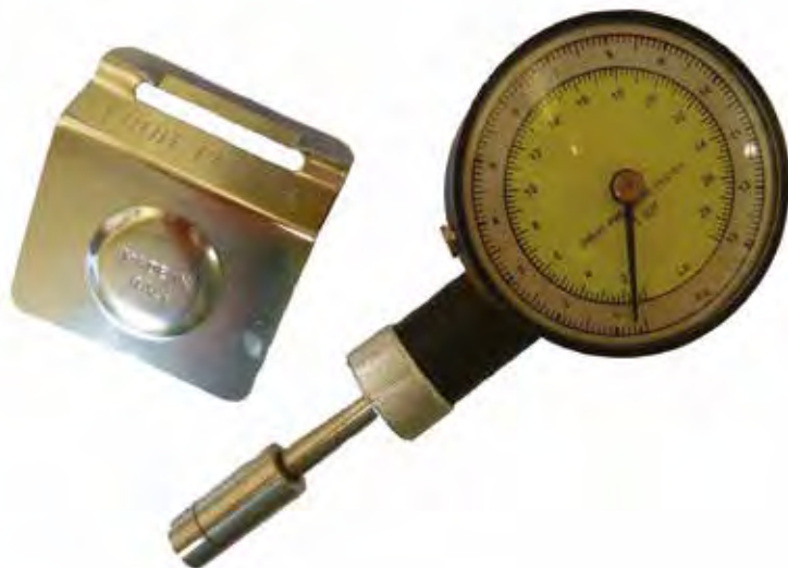
Figure 20. Hand-held penetrometer for measuring fruit firmness.
