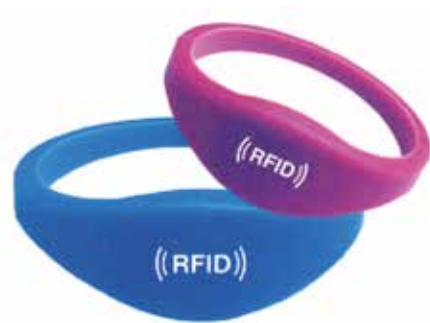
Figure 28. Radio frequency identification (RFID) wrist bands.
