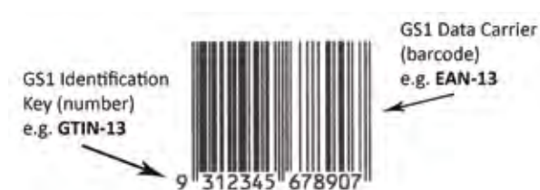
Figure 44. An example of a barcode (not to scale).
