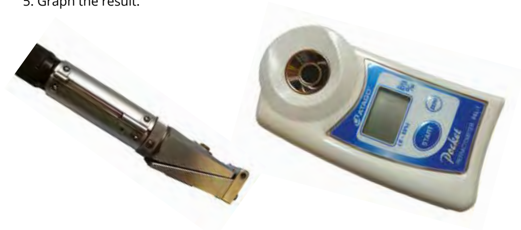
Figure 21. Hand-held and digital refractometers for measuring fruit soluble solids content
