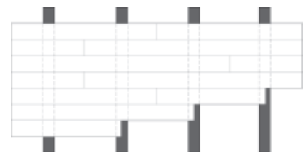
Fig.2. Butt joints for end matched boards.
