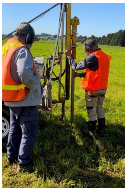
Soil core sampling at TDRF. Photo by Adam Langworthy.
