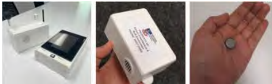
Figure 1: Data logger and survey tablet (left); the node (centre); iButton (right)
