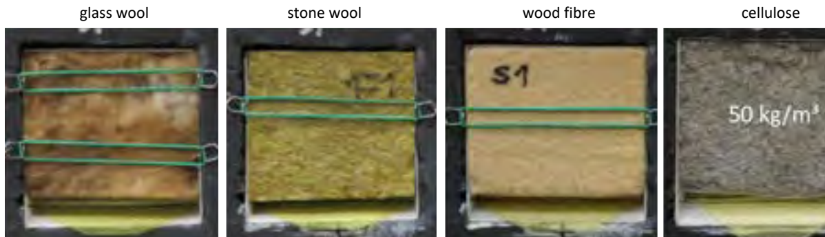
Figure 38: Mounting of insulation materials on condensation test equipment.
