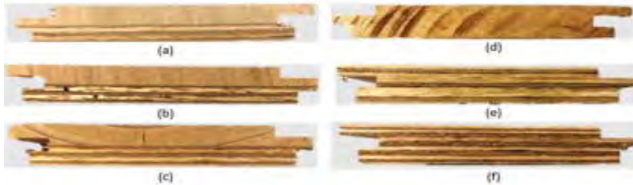
Figure 2: Cross sections of the developed flooring prototypes (a-c: 6 mm plantation E. nitens on marine plywood substrates, d: solid densified E. nitens , e: 1.2 mm E. nitens veneer on marine plywood, F: 1.2 mm E. nitens veneer on E. nitens plywood)
