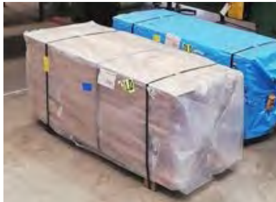
Figure 2. Clear and Opaque wrapped timber in-situ
