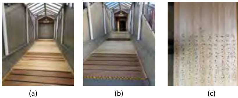
Figure 3: In-service trials and testing of flooring prototypes ((a) solid flooring trial, (b) engineered flooring trial, (c) dynamic hardness test conducted on an engineered flooring prototype)
