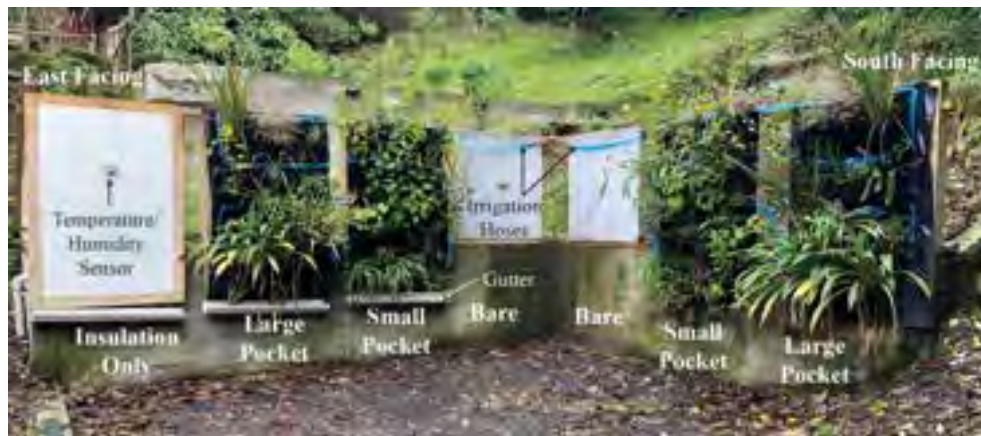
Figure 2: The experimental living wall setup in Wellington, Aotearoa New Zealand, in February 2023. The bare walls act as controls for orientation and are used to compare the effects of the living walls. (Source: Author)
