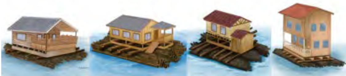
Figure 3: Illustration of the types of floating houses in Agusan marsh (from left to right – type 1 - hapa, type 2 - hanger, type 3 - hapa-hanger combination, and type 4 - dos andanas)
