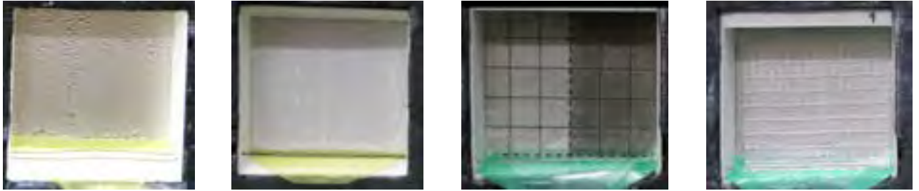
Figure 36: Tested surface samples from left to right: metal (hydrophilic), PE film (hydrophobic, smooth), film laminated on fleece (hydrophobic, fine structured), film reinforced with fabric (hydrophobic, coarse structured).
