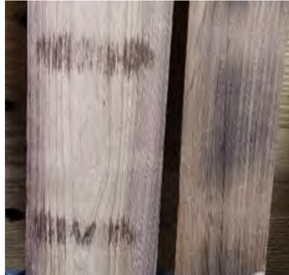
Figure 10 - Blackwood timber displaying left to right - dark sticker marks, light sticker marks.
