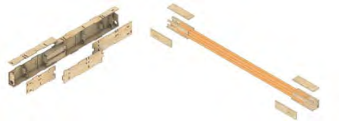
Figure 32: Bearer comparison - initial design (left) and final simplification (right).
