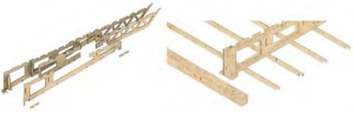
Figure 33: Exploded view of a typical beam (left); connection to the ceiling battens (right).
