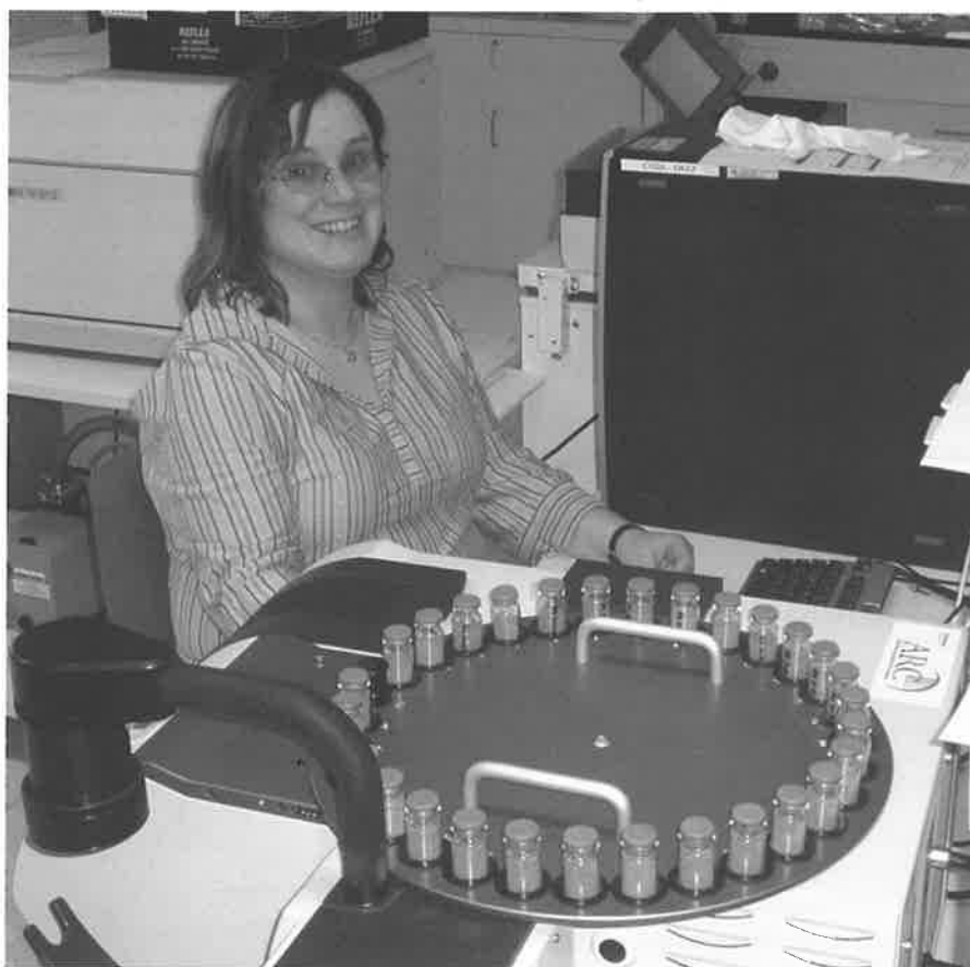
Linda Ballard analysing wood samples for cellulose and lignin using the NIR analyser.
