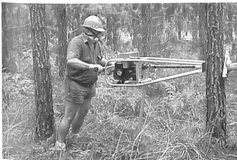
Dr Kevin Harding sampling six-year-old F 1 slash x Caribbean pine hybrids using QFRI locally developed motorised increment corer, MASTA (Motorised Apparatus for Sampling Trees for wood Assessment).
