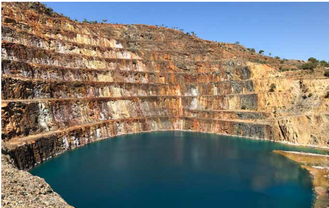
Uncovering Northwest Queensland's hidden potential: Mary Kathleen open pit, NW Queensland, looking southeast. Uranium is contained in thin, shallowly dipping veins cutting through the host rock.
