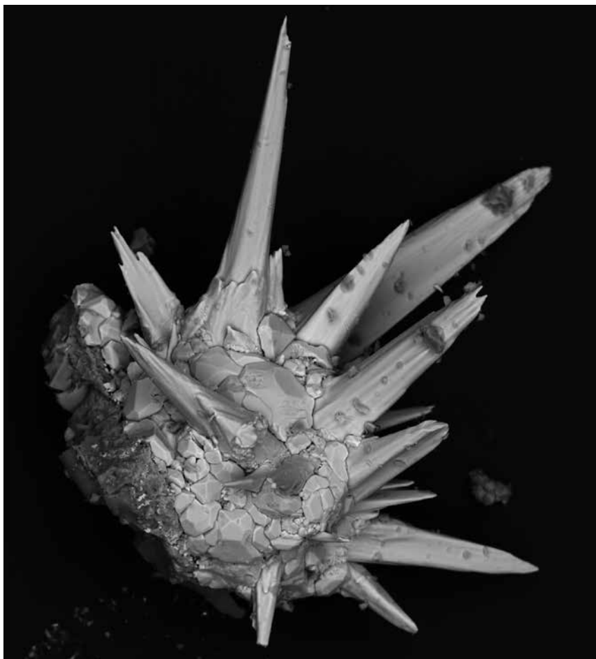
This image shows the products of reaction (cuprospinel, hematite and tenorite) between hot gases and solidifying magma in the lava tube of the 2013 Tolbachik eruption, seen under magnification. It was published in 2018 in the journal Minerals as part of Vadim Kamenetsky's contribution to an article on the 2012–2013 eruption of the Tolbachik Volcano in Kamchatka, Russia.
