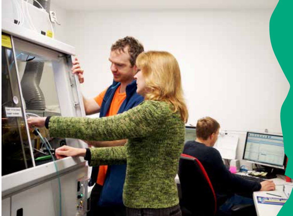
Jeff Steadman and Irina Zhukova inspect the sample chamber of an LA-ICP-MS at CODES, while Aleksandr (Sasha) Stepanov (seated) programs a series of LA-ICP-MS analyses.
