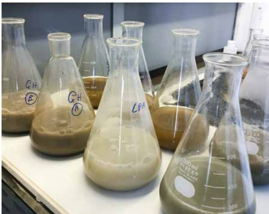
Accelerated hydrogen peroxide testing on mine waste materials conducted as part of an ATSE-funded project led by Dr Anita Parbhakar-Fox on improving column feed characterisation prior to kinetic testing.
