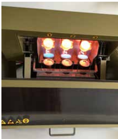
Fusion of rock powders mixed with borate flux at ~ 1000°C using CLAISSSE M4 FLUXER TM during sample preparation for chemical analysis of rocks via X-ray fluorescence (XRF). The melt is released into a flat mould and, after cooling, results in a glass disk ready for XRF analysis of major chemical constituents.
