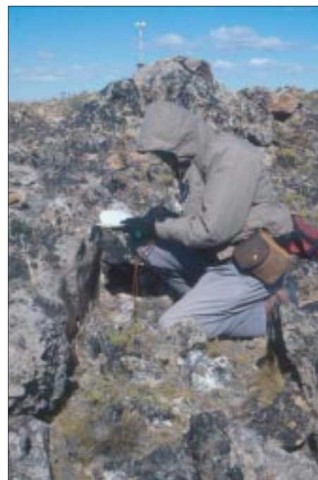
Robert Scott measures fault striations developed along the Concepcion Vein, Cerro Vanguardia (48°S), Argentina.
