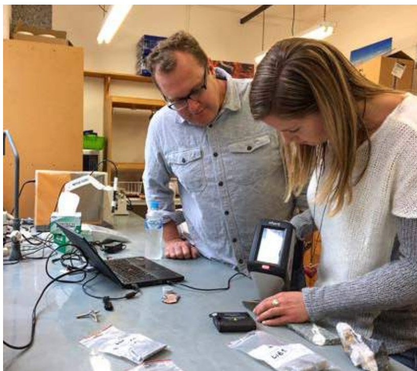
ABOVE: PhD student Laura Jackson with Andrew Somers from SciAps testing a portable laser-induced breakdown spectroscopy (PLIBS) device for rapid chemical analysis of waste rock samples.
