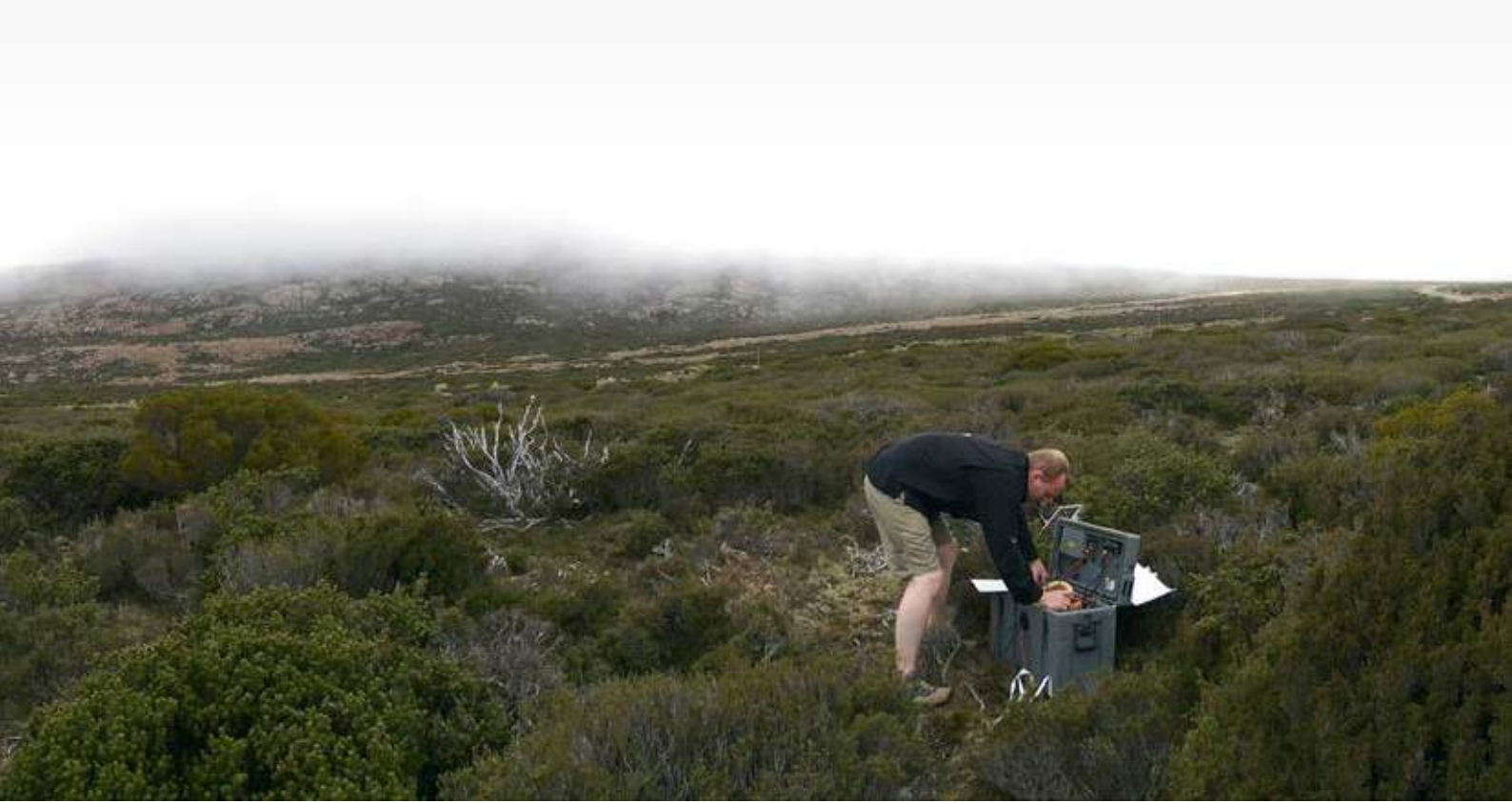
ABOVE: PhD student Matthew Ferguson deploying an MT instrument on Ben Lomond plateau, northeast Tasmania. Matthew was assisting PhD student Tom Ostensen, who is using the data to learn more about Tasmania's crustal structure as part of CODES' Program 6 research.
