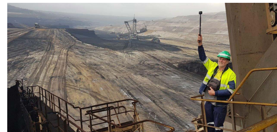
Hambach lignite mine, Germany. Dr Michael Roach taking 360-degree imagery on a bucket-wheel excavator in the open pit. Bucket-wheel excavators, like the ones in the background, are used for soft rock overburden removal and lignite mining. The imagery collected by Michael is being used to create a virtual tour of the mine.
