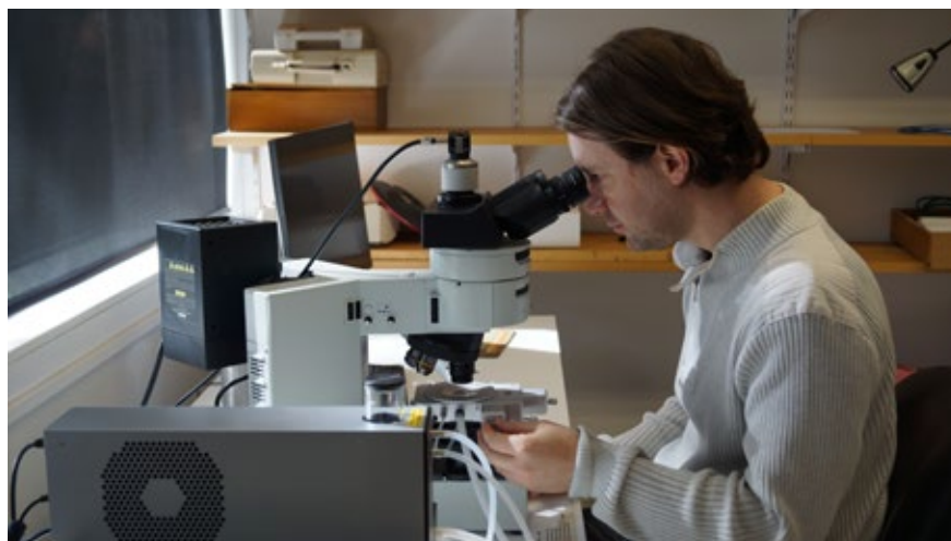
Dr Francisco Testa locating CO 2 -rich fluid inclusions in quartz prior to microthermometric measurements.
